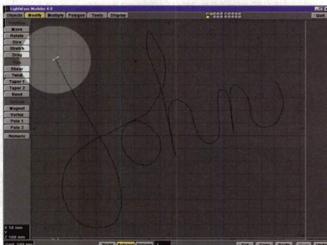
Figure 1: Make sure you align your flat disc to the start of the curve you'll use for Rail Extrude.
